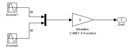
The input to the timestwo S-function comes from two arrays located at two different memory locations, one for the output of sourcel and one for the output of block sourcel. This is because of an optimization that makes the Mux block virtual, meaning that code is not explicitly generated for the Mux block and thus processor cycles are not spent evaluating it (i.e., it becomes a pure graphical convenience for the block diagram). So this is represented in the *model*.rtw file in this case as
